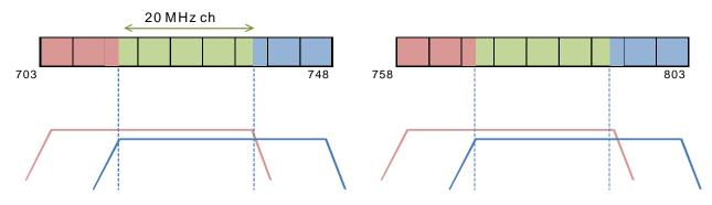
Figure 11. 20 MHz channel in the middle of the band
