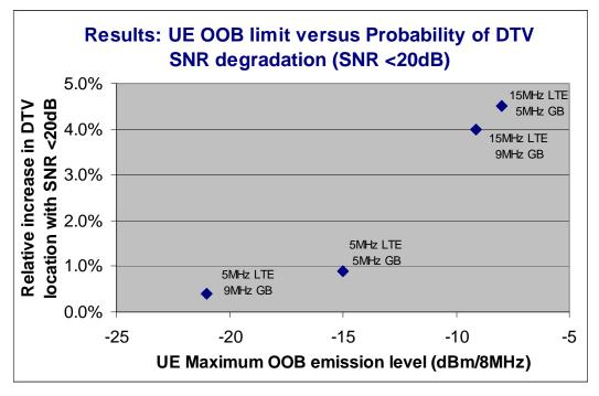
Figure 7. UE OOB limit versus probability of DVB SNR degradation < 20dB
