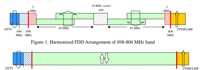
Figure 2. Harmonised all-TDD Arrangement of 698-806 MHz band
