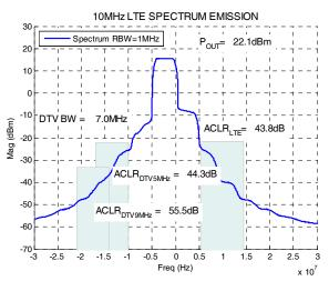
Figure 10. ACLR for partial band allocation (25 RBs, offset 0) to UE
