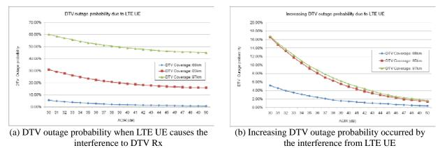
Figure 5. DTV outage due to the interference of 10MHz LTE UE
