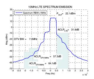
Figure 9. ACLR for partial band allocation (25 RBs, offset 25) to UE
