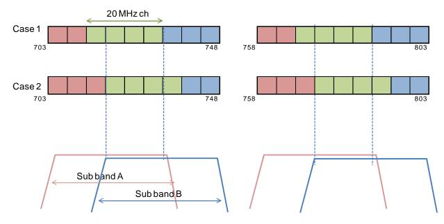
Figure 12. 20 MHz channel positions with 5 MHz raster
